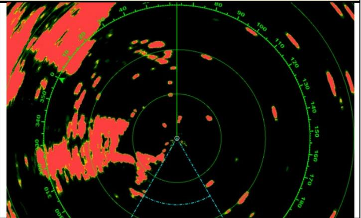
These images are from the area around the Kobe Airport in the 3 NM range scale. The DRS2D-NXT in Target Analyzer helps intuitively identify approaching and stationary targets around the airport.
