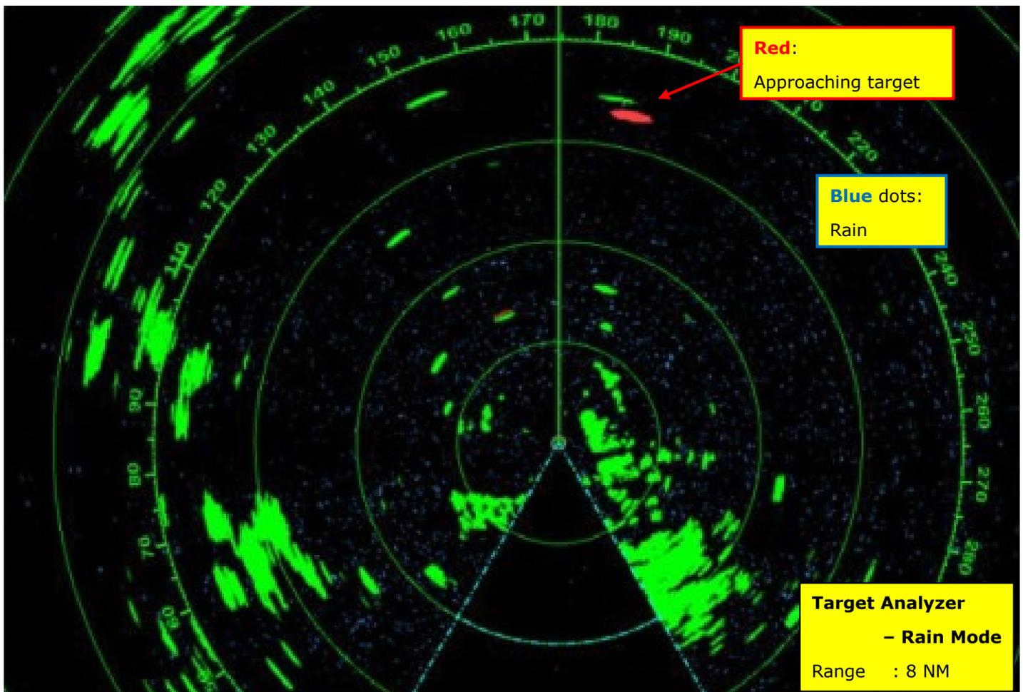
**Note:** The DRS2D-NXT has a wider beam than the other models due to a shorter antenna length: Rain clutter is smoothed, so that rain targets are shown in weaker dots than would be shown on other models.
