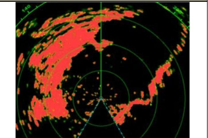
The DRS2D-NXT shows similar images to the DRS4D-NXT in a long range scale of 24 NM. Due to the longer antenna, bearing resolution is superior with the DRS4D-NXT: The DRS4D-NXT shows echoes more sharply than the DRS2D-NXT.
