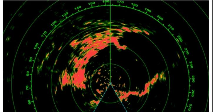
These screenshots show Osaka Bay in the 24 NM range scale. The Solid-State DRS2D-NXT is compared with the magnetron-type DRS4DL+; the DRS2D-NXT shows clearer coastlines inside Osaka Bay.
