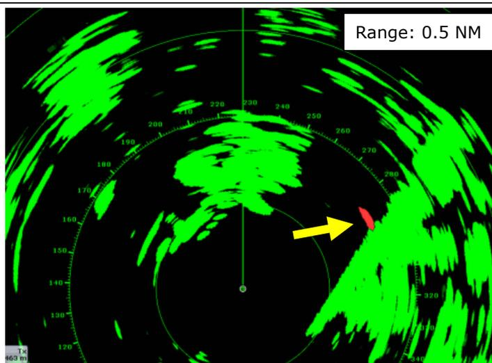
This target is located alongside a wharf. In the conventional presentation mode, this target will be shown in the same color as the wharf and can be interpreted as a part of the wharf structure. Target Analyzer helps identify the approaching target shown in red.
